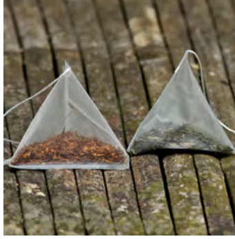
Figure 4.1: Tetrahedron-shaped synthetic tea bag used for TBI experiments.
